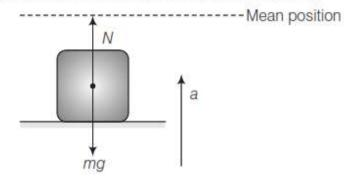
It is accelerating towards mean position that is vertically upwards. Writing equation of motion
