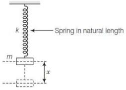
Suppose x is the maximum extension in the spring when it reaches the lowest point in oscillation.
