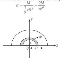
(a) The half-disc can be supposed to be consists of a large number of semicircular rings of mass dm and thickness dr and radii ranging from r = 0 to r = R.
