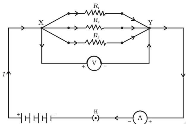
Figure 11.7 Resistors in parallel
