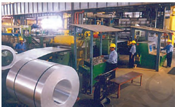
Fig. 6.3: Strip coating mill at smelter of NALCO
